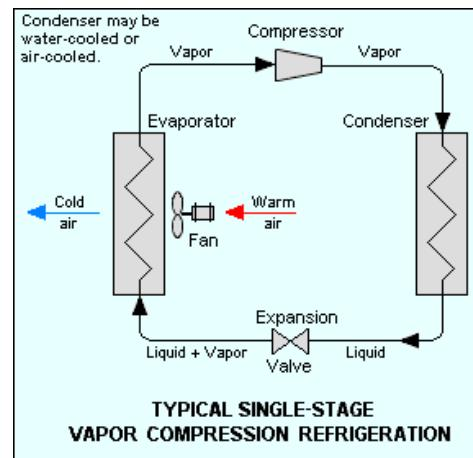
**Vapor compression cycle with increase in pressure and temperature of evaporator and decrease in condenser pressure and temperature**
